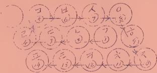
The most frequently used letters are losted toward the center of the middle brak; and the least used letters are pushed into the corner of the bottom line.
